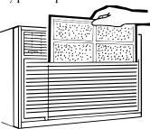
Remove the 2 screws and lift off the front grille. Keep these screws to re-attach the grille later.
